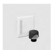
**Built-in wall box with ventilair® air-admittance valve DN 30-50** Box dimensions w x h x d =  $130 \times 150 \times 93$  mm, suitable for brick wall and drywall installation, box depth adjustable by maximum 65 mm, mounting frame for cover plate, polystyrene protection block, plastic cover plate, UV resistant, w x h =  $165 \times 190$  mm, alpine white
