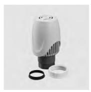
**ventilair duplex® two-way vent valve G 1 1/2 DN, 40/50** Volume flow 8 l/s, temperature range -20°C to +60°C, with activated carbon filter, polystyrene frost protection cover
