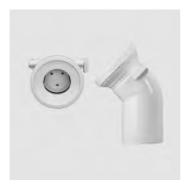
WC connecting bend 45°, DN 100, with lockable rat blocker In white PP plastic, for floor-standing WCs, with built-in mechanical rat blocker, rear side of valve clad with bite-resistant stainless steel, prevents the invasion of foreign objects to the WC, additional manual operation for cleaning by
